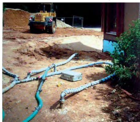
Fig. 2: ThermoAir test field at a CHC spill site nearby Frankfurt (three insulated 2" injection tubes and one extraction well in center)
