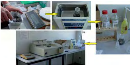
Figure 3: Fast detection of PAH in soil
