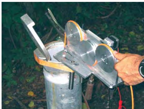
Figure 11: Cable winch with 12 V DC motor
