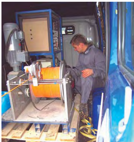
Figure 9: The early 220 volt cable winch
