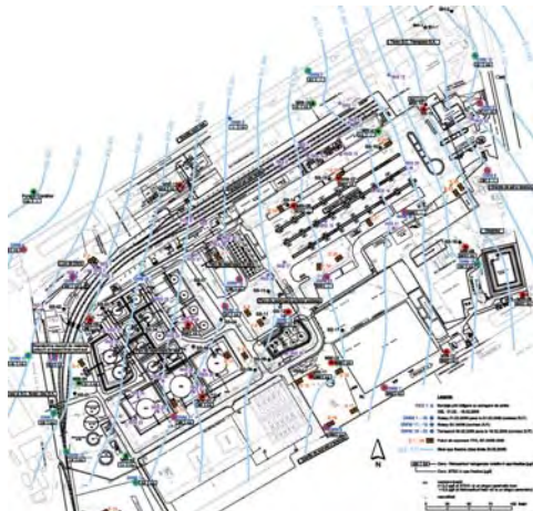
Figure 6: BTEX-concentration in groundwater
